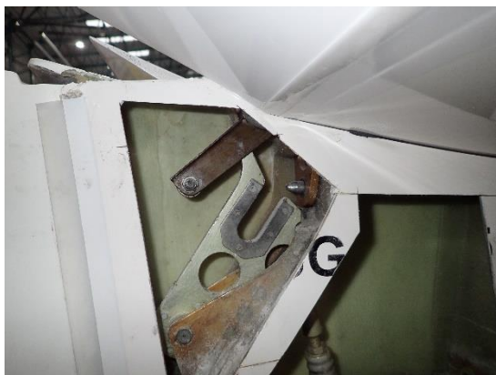
Disconnected elevator control
